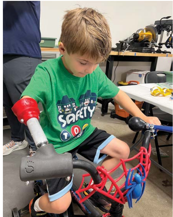
A Form5 Bike Arm Adapter recipient tries out his new prosthetic device.
